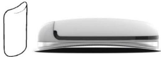
Figure 10: Illustration of Gemperle's humanistic form, juxtaposed with the pump's side-view, showing its concave base.
